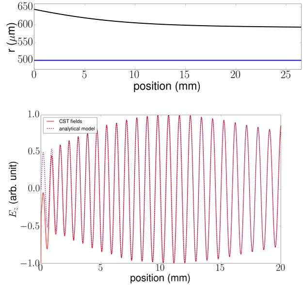
Figure 1: The tapered structure in our example for a fixed inner radius  $a=0.5$  mm (blue) and a tapered Quartz ( $\epsilon_r = 4.41$ ) dielectric thickness with outer radius (shown red). The taper is matched for an initial energy of  $\mathcal{E}_i=205$  keV with a maximum accelerating field of  $E_0=100$  MV/m. We show the comparison with CST-MWS (bottom) for completeness.
