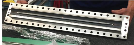
Figure 5: Picture of the top assembly of the stripline kicker, showing the copper stripline electrode and the stainless body which have been coated and treated to increase the emissivity.
