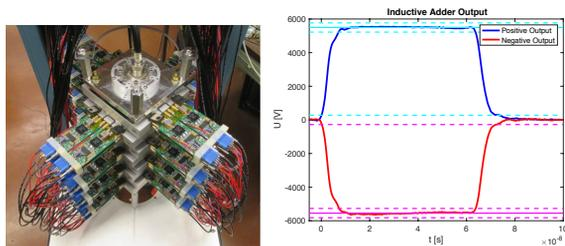
Figure 3: (Left) Full assembly (8 stages) of inductive adder. (Right) Voltage output of inductive adder at 105% of nominal setpoint.
