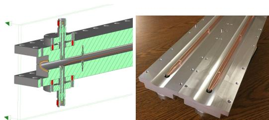
Figure 4: (Left) CAD model of stripline kicker with small gap and tapered electrodes. (Right) Prototype of stripline kicker.
