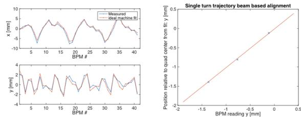
Figure 9: (Left) First turn trajectory of injected beam in the ALS - intentionally launched off-axis in the vertical plane – as well as trajectory fits using the ideal machine model. (Right) beam based alignment measurement for one quadrupole with the result agreeing within 50 microns with stored beam beam-based-alignment measurement.
