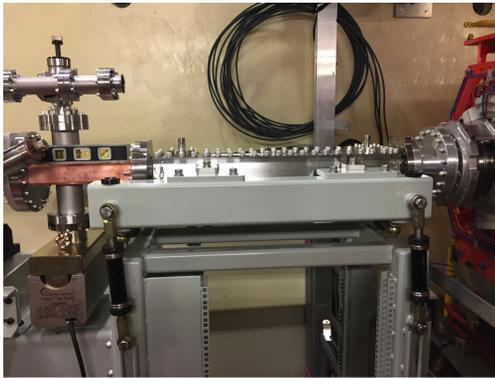
Figure 7: Stripline kicker with 6 mm full aperture between the striplines installed in the ALS.
