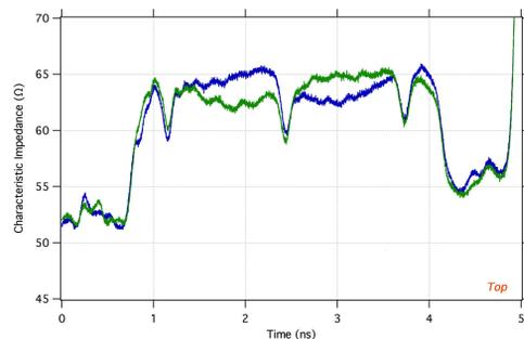
Figure 6: TDR measurements of the top and bottom striplines of the kicker. In the measurements, only one electrode is excited. The nominal impedance for that case is about 64 Ohms.
