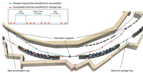
Figure 2: Illustration of the planned swap-out process between the full energy accumulator and the storage ring of ALS-U.
