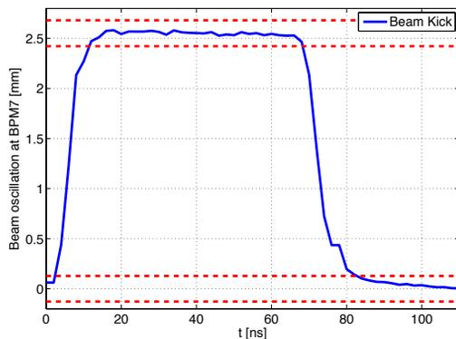
Figure 8: Full beam test mapping the beam integrated kick with turn-by-turn BPMs for the stripline kicker and pulser installed in the ALS.
