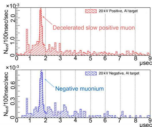
Figure 3: The top figure shows the TOF distribution of the decelerated positive muons. The bottom figure shows the TOF distribution of the negative muonium.
