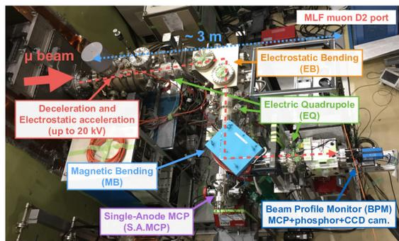
Figure 2: The diagnostic beam line for the LE muon beam using the metal foil target.
