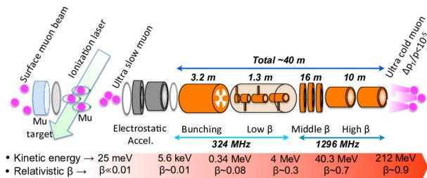
Figure 1: The conceptual diagram of the muon linac.
