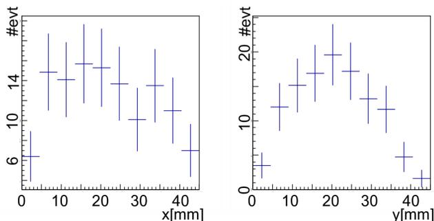
Figure 4: The projections of the beam profile of the LE positive muons decelerated by the thin metal foil. The left and right figures are for the horizontal and vertical direction, respectively. [The projections were corrected based on the geometric shape of the LE BPM. The error was only the statistical error based on Poisson distribution.]
