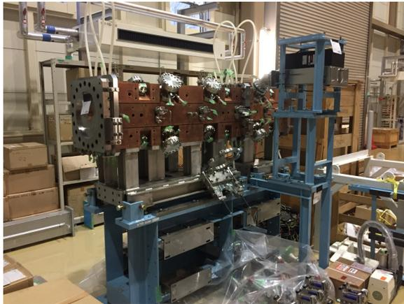
Figure 5: J-PARC linac prototype RFQ.
