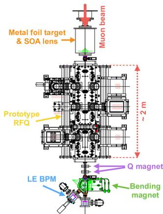
Figure 6: The latest drawing of the muon acceleration test using the prototype RFQ at the muon D line.
