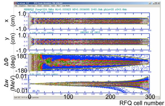
Figure 7: The particle tracking simulation of the prototype RFQ assuming the  $\text{Mu}^-$ .
