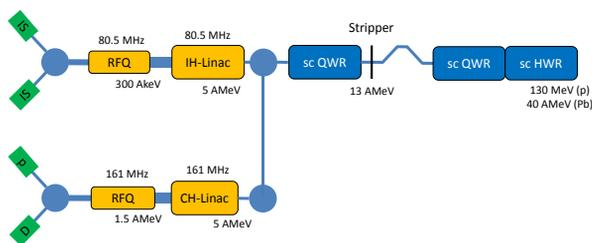
Figure 1: Conceptual layout of the hadron driver linac with two front-ends.
