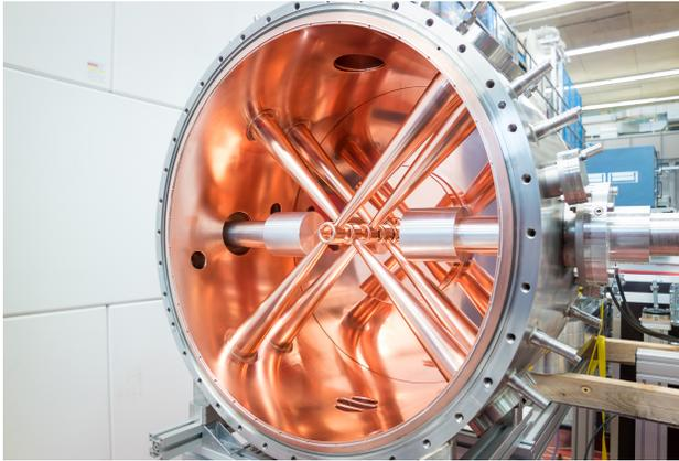
Figure 5: CH-cavity for the FRANZ Linac that is similar to the first CH-cavity of the light ion front end.
