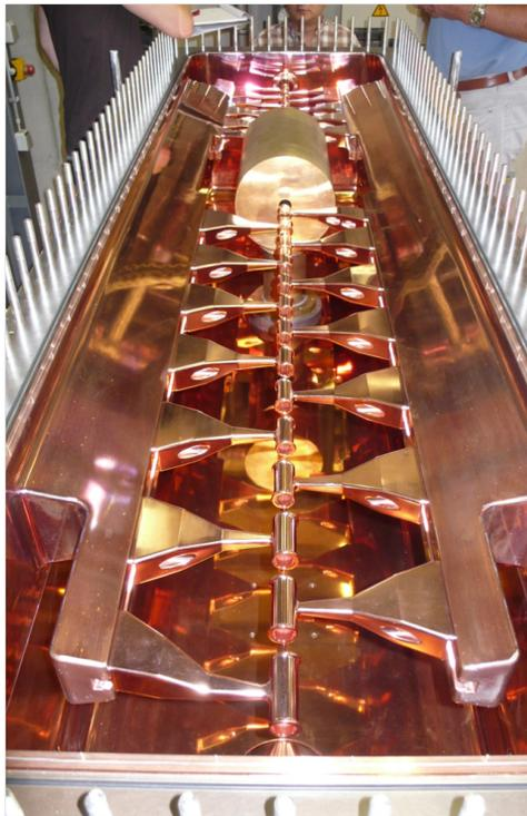
Figure 3: IH-cavity of the BNL EBIS Linac is very similar to the first IH-cavity of the heavy ion front-end [4].
