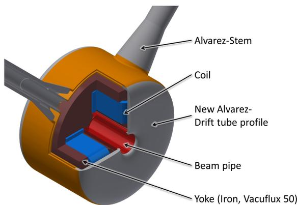
Figure 6: CAD-model of the drift tube with the new shape profile and an integrated quadrupole singlet. The first and shortest drift tube has a total length of 111.3 mm, an aperture of 30 mm, and its diameter is 180 mm.
