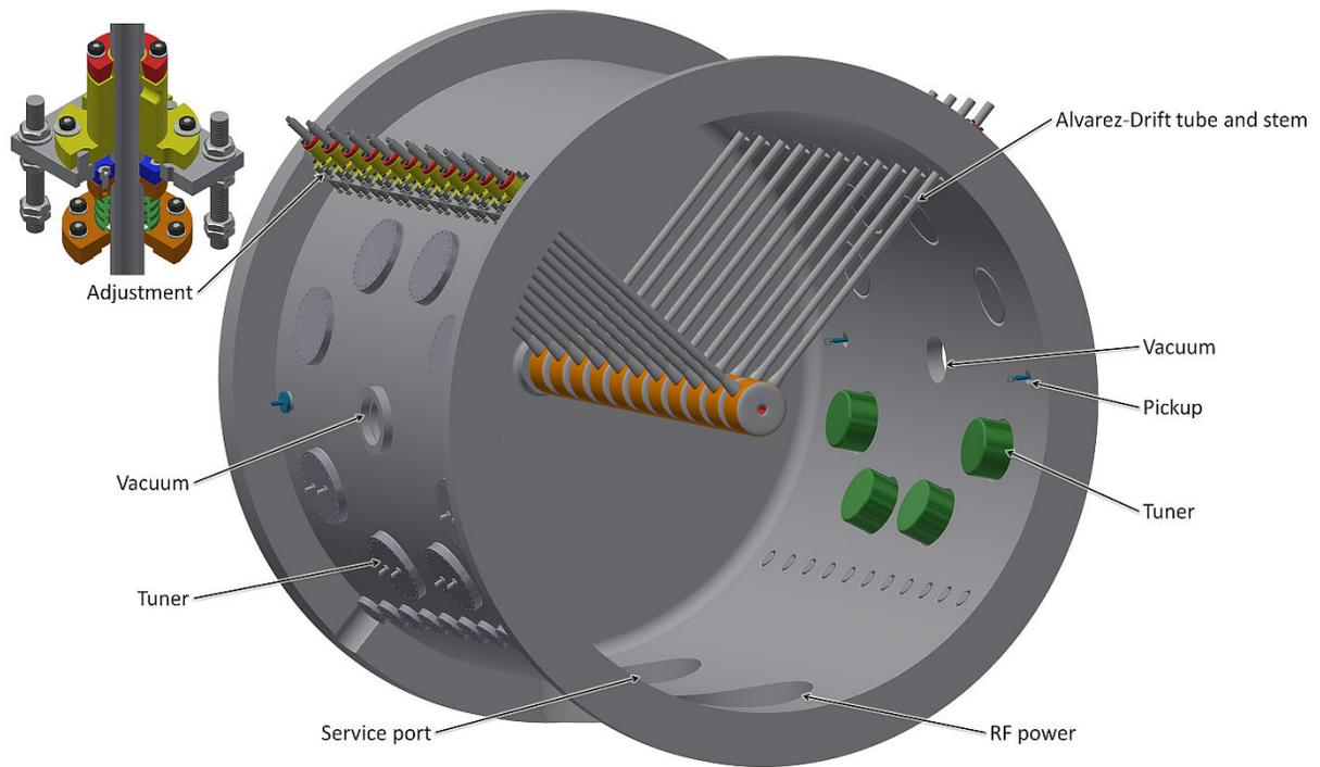
Figure 3: CAD-model of the Alvarez-prototype cavity section with a length of 1.9 m and 11 drift tubes. The drift tubes are installed at the top of the tank, but other combinations can be installed. The bottom houses RF coupling, a support hole, and at the side the vacuum pumps and pickups are installed (blue).
