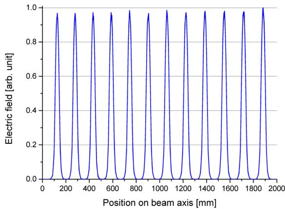
Figure 5: Simulated electrical field distribution on beam axis at 108.4 MHz for the Alvarez-prototype.
