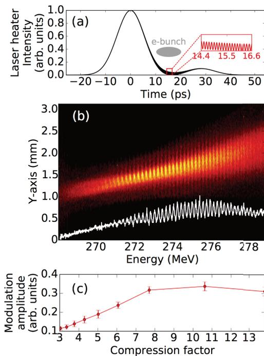
Figure 2: (a) Theoretical LH laser pulse, (b) electron beam spectrometer image and energy spectrum (white line), and (c) amplitude of the energy modulation (white line in b) versus compression factor. The LH parameters are: central wavelength = 780 nm, bandwidth = 8.4 nm (FWHM), pulse duration = 12.9 ps (FWHM), delay = 28.2 ps.
