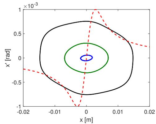
Figure 2: Matched beam after ten turns. Initial ellipses exhibit different angles, depending on whether particles see a positive or a negative self-field gradient and the respective incoherent tune-shifts.
