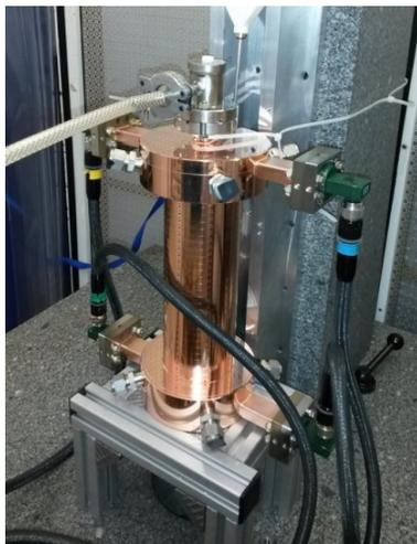
Figure 2: Structure ready for vertical bead-pulling.
