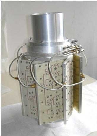
Ring slot-coupler RF structure (design FZJ)
