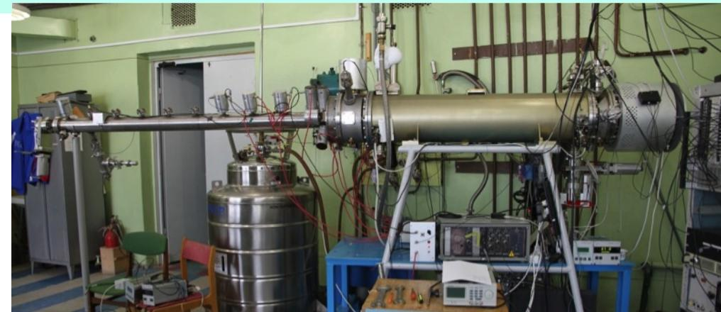
B= 5.4T reached. Test Au beams produced:
