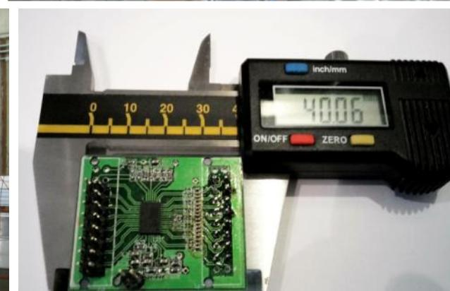
**Readout Electronics developed for TPC,
