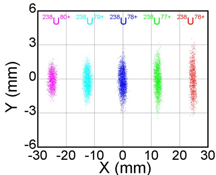
Uranium ion beams with various charge states after charge selection slits
