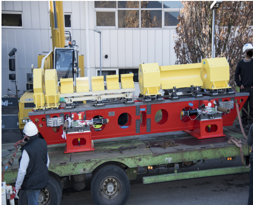
Girder prototype with dummy magnets: Mechanical tests
