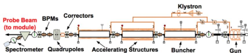
Figure 1: The CALIFES beam line, as installed in the CLIC Test Facility 3
