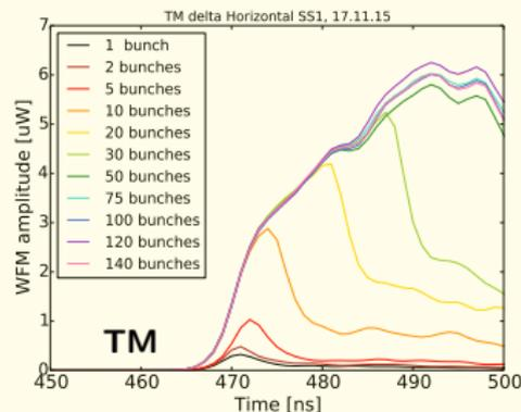
Signal buildup until steady-state depending on the number of bunches (0.17 nC per bunch)
