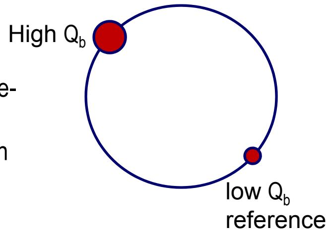
Need good resolution at low current, and many BPMs capable of resolving the orbits of at least two bunches
