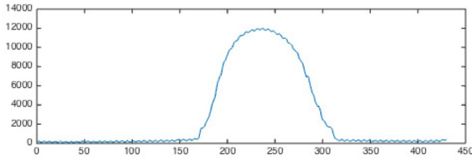
Beam profile is acquired on the second profile monitor prior insertion of the slits for the emittance measurement. Beam charge is 1 nC.
