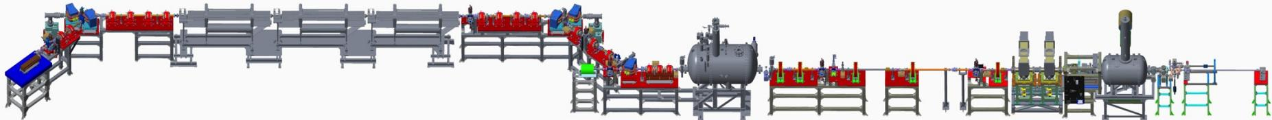
Electron beam is generated by 113 MHz SRF gun with photocathode driven by a 532 nm laser. Two 500 MHz copper cavities provide energy chirp and beam is compressed to desired peak current. After compression beam is accelerated by a 704 MHz SRF cavity and merged into CeC PoP structure having three helical undulators.
