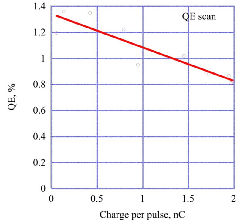
The photocathode was excited with 1 nsec laser pulse with varied optical energy. Gun voltage was 1.2 MV and laser spot size 1 mm r.m.s.
