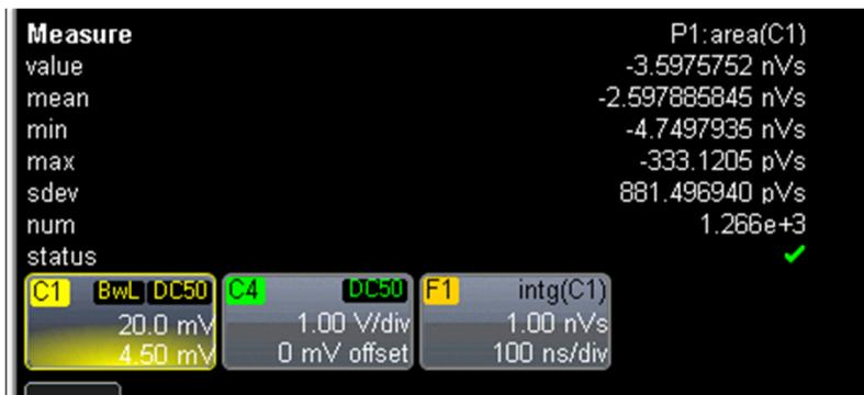
First beam was observed in 2015 with integrating current transformer during phase scan. The charge was 0.5 nC.
