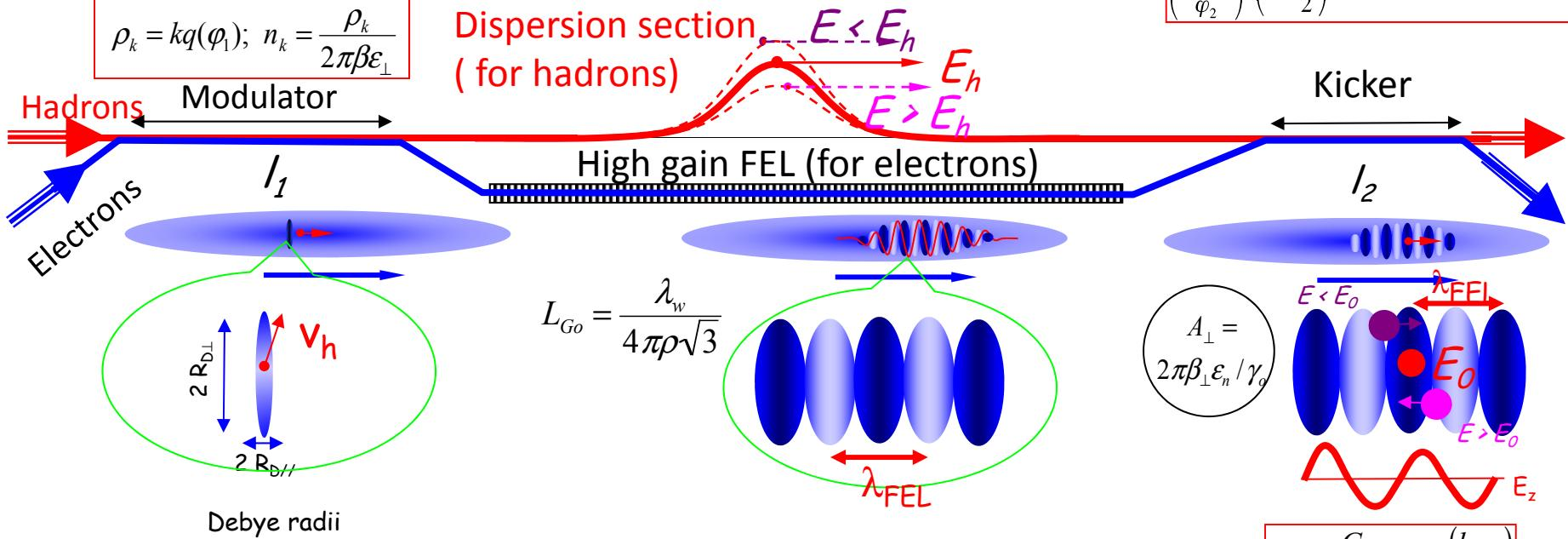
Amplifier of the e-beam modulation in an FEL with gain  $G_{FEL} \sim 10^2 - 10^3$
