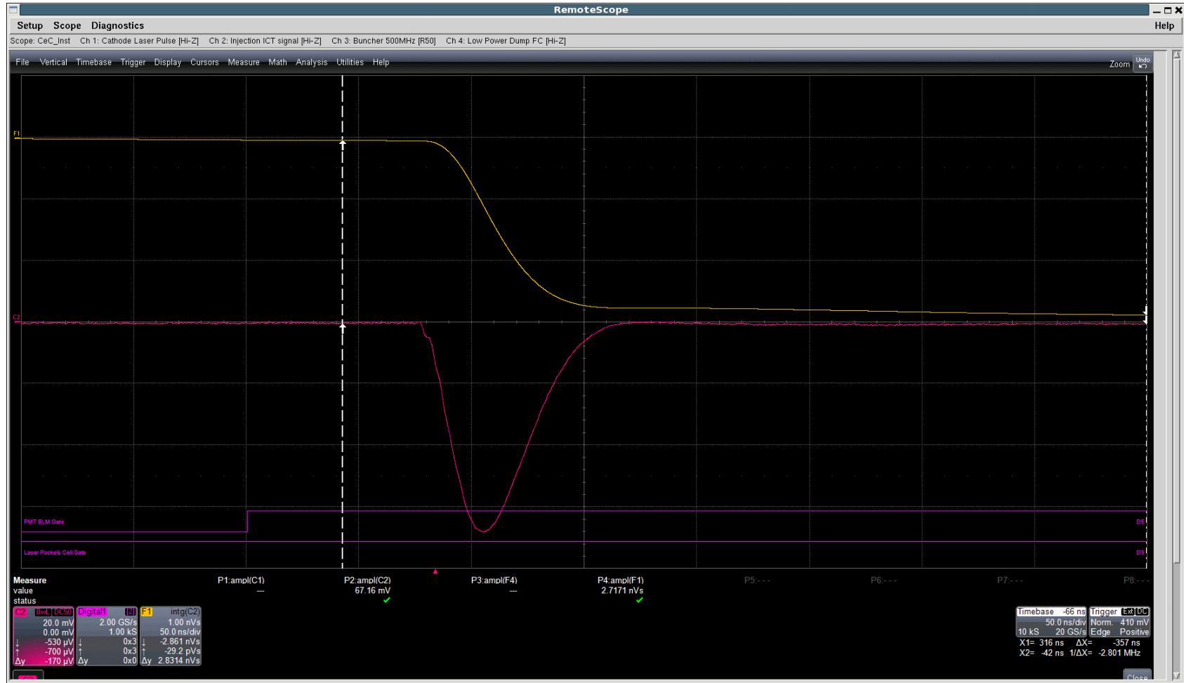
Beam was excited with 1 ns laser pulse with 0.5  $\mu$ J energy. 2.7 nVs ICT voltage integral corresponds to 2.1 nC charge. On the second day cathode was demonstrating 1 nC charge (100 pC at the end of the week).
