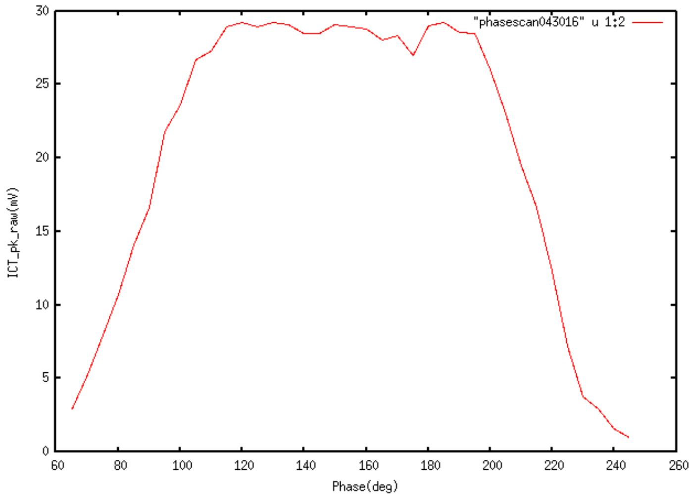
Cavity phase scan is consistent with last year measurements and simulations.
