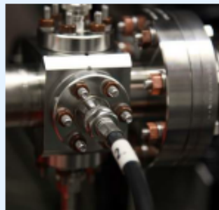
BPM Installation in FLASH
