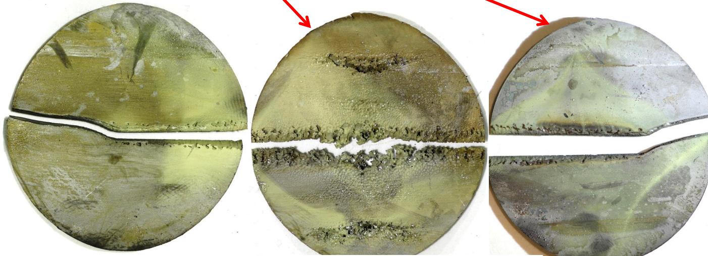
Cavitation damage to target inner wall
