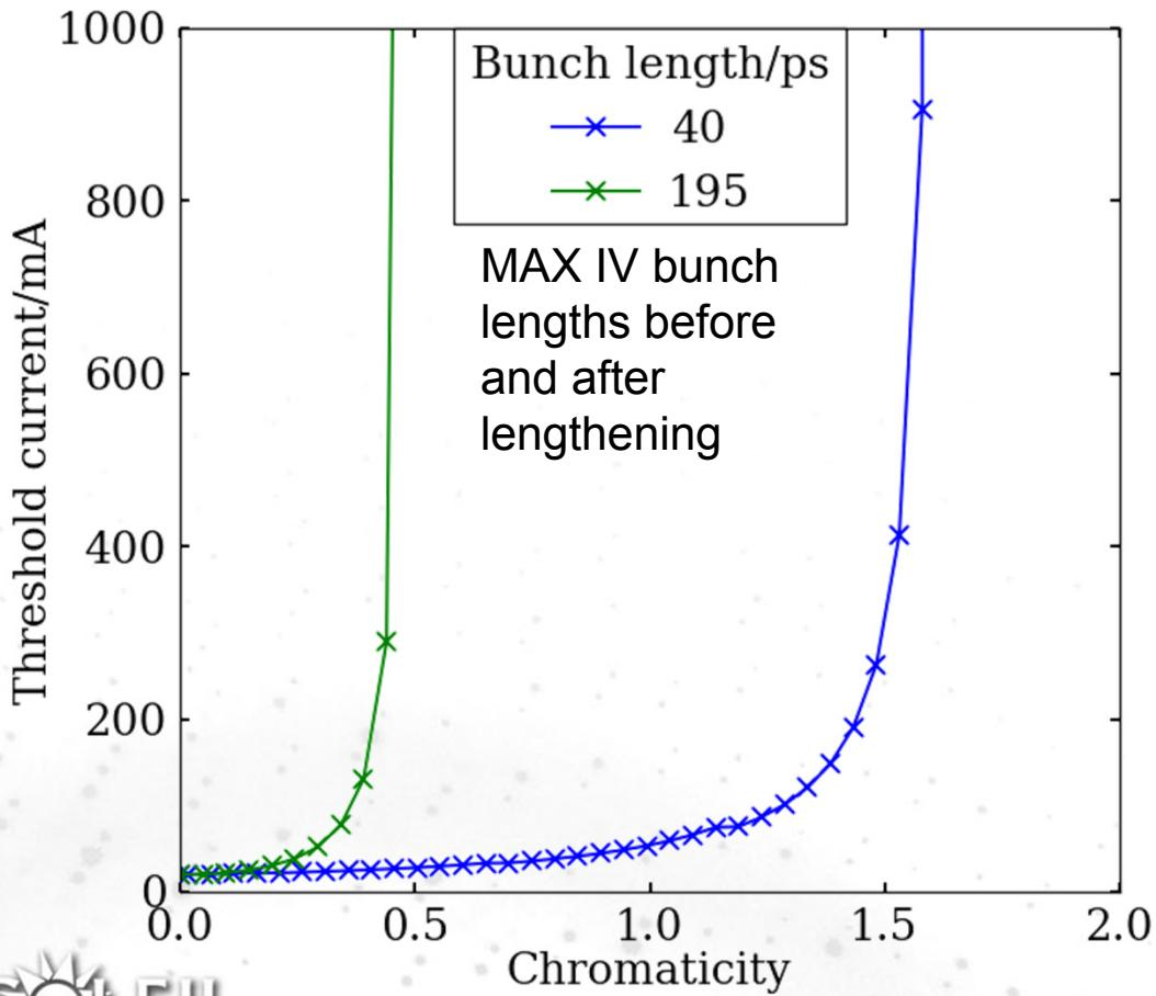
With positive momentum compaction, a positive chromaticity stabilises beam against resistive wall impedance
