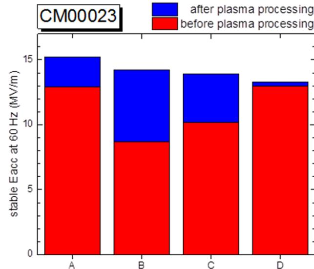
Performance improvement for the four cavities in cryomodule after in-situ plasma processing.
