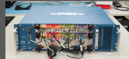
XFEL/PSI Modular BPM Unit for both button and cavity BPMs. (courtesy B. Keil)
