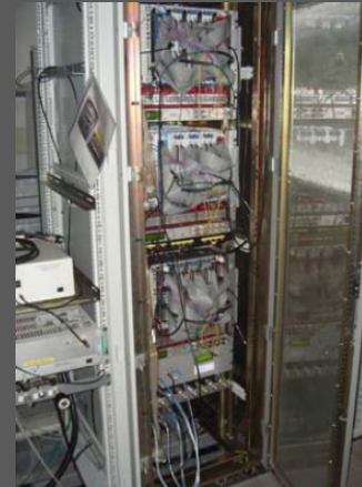
Elettra (SLS) longitudinal and transverse processors: VME implementation
