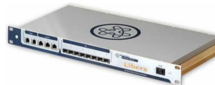
ESRF, Diamond, Alba, NSRRCC, CLS, ANKA, ALS longitudinal/transverse feedback processor (Libera bunch by bunch by Instrumentation Technologies)
