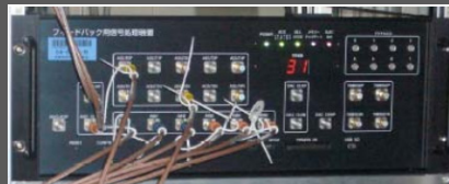
Spring-8 transverse feedback processor (adopted by TLS, KEK-Photon-Factory and SOLEIL)
