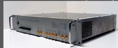
DAΦNE (transverse), KEK-Photon-Factory (longitudinal), ALS, DELTA, Indus-2, NSLSII, SPEAR3 feedback processor (iGp by Dimtel)
