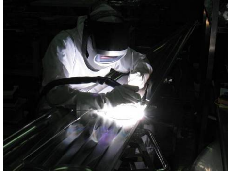
Welding pumping port
