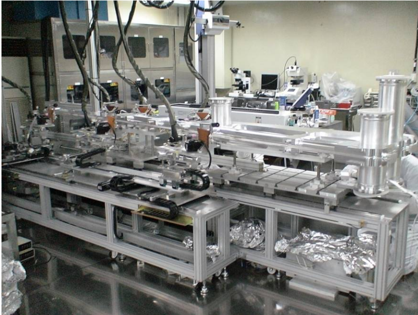
Bending chamber in auto-welding stage
