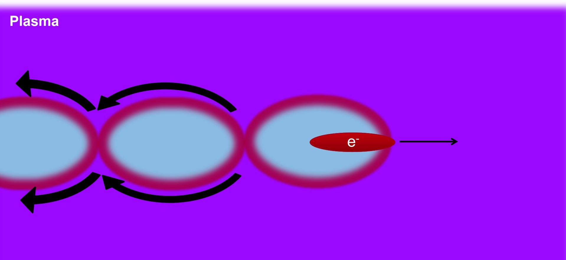
The plasma electrons keep oscillating after the beam has passed by.
