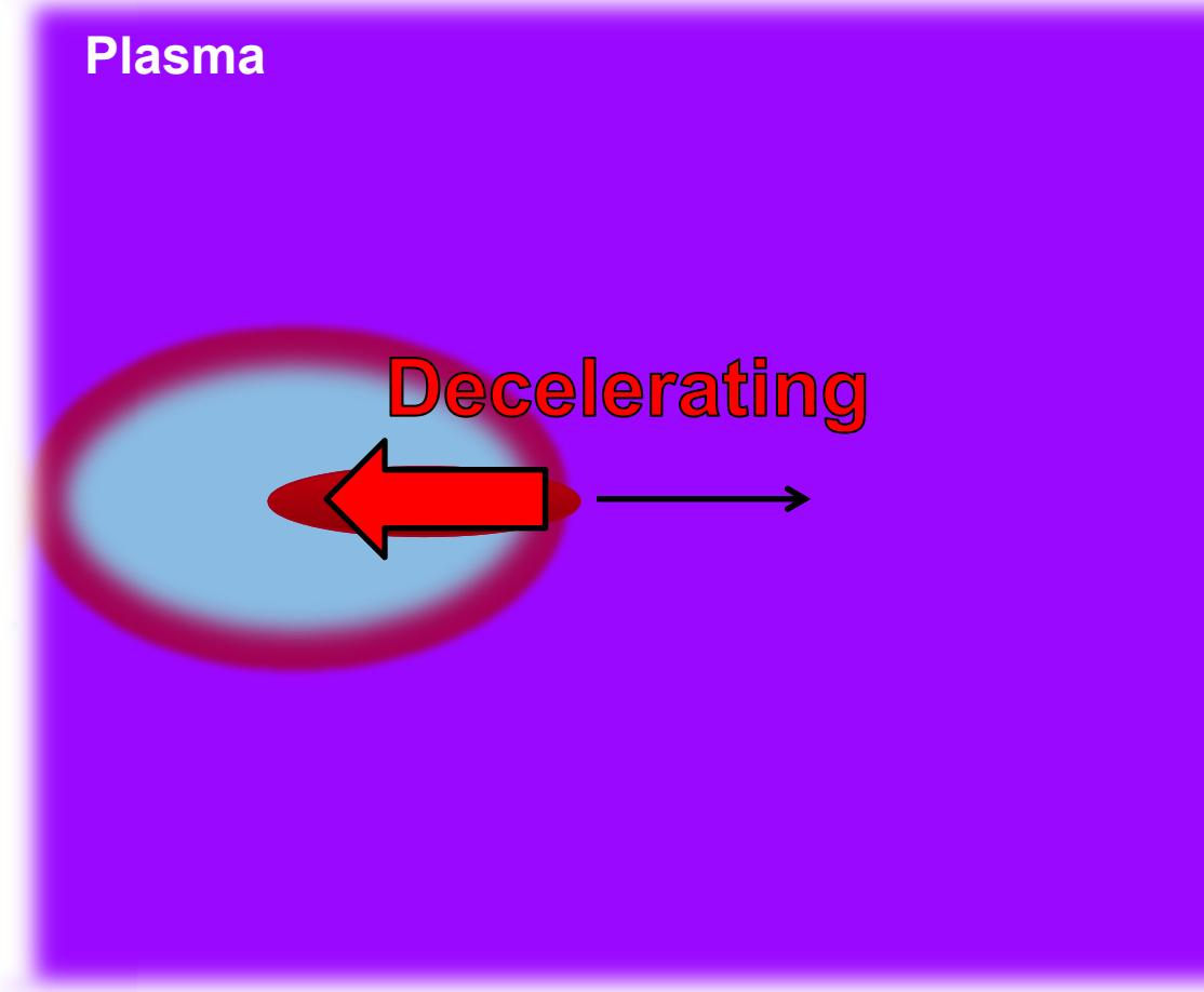
The field is **decelerating** in the front half of the bubble. The plasma extracts energy from the electron beam.
