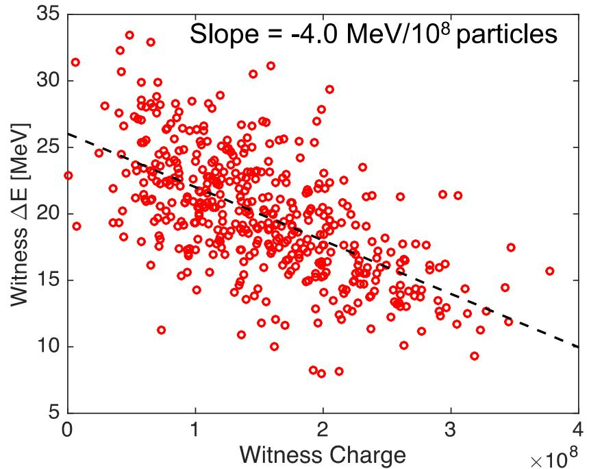
Beam loading is an important consideration when trying to optimize the gradient and efficiency. The average drive-to-witness efficiency in this experiment was 18%.
