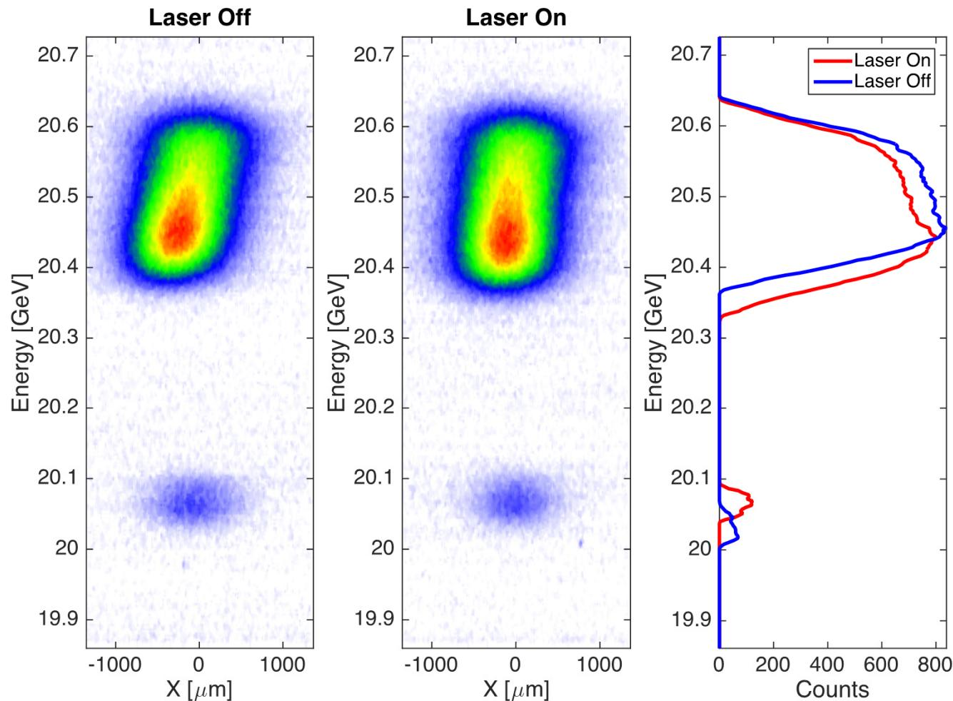
Energy gain of up to 33.4 MeV in 25 cm long channel!
