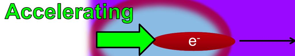
The field is **accelerating** in the back half of the bubble. Beam electrons can extract energy from the plasma wake in this region.
