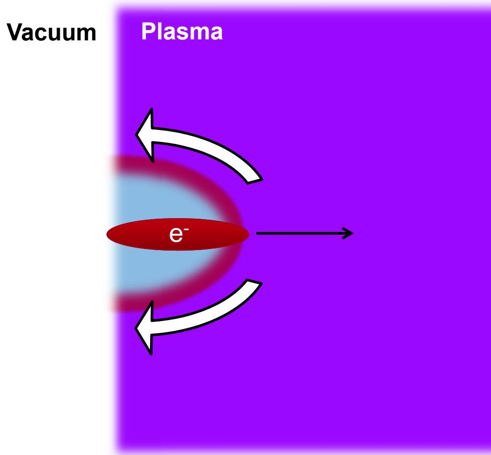
As the beam enters the plasma, plasma electrons are expelled, leaving behind plasma ions.
