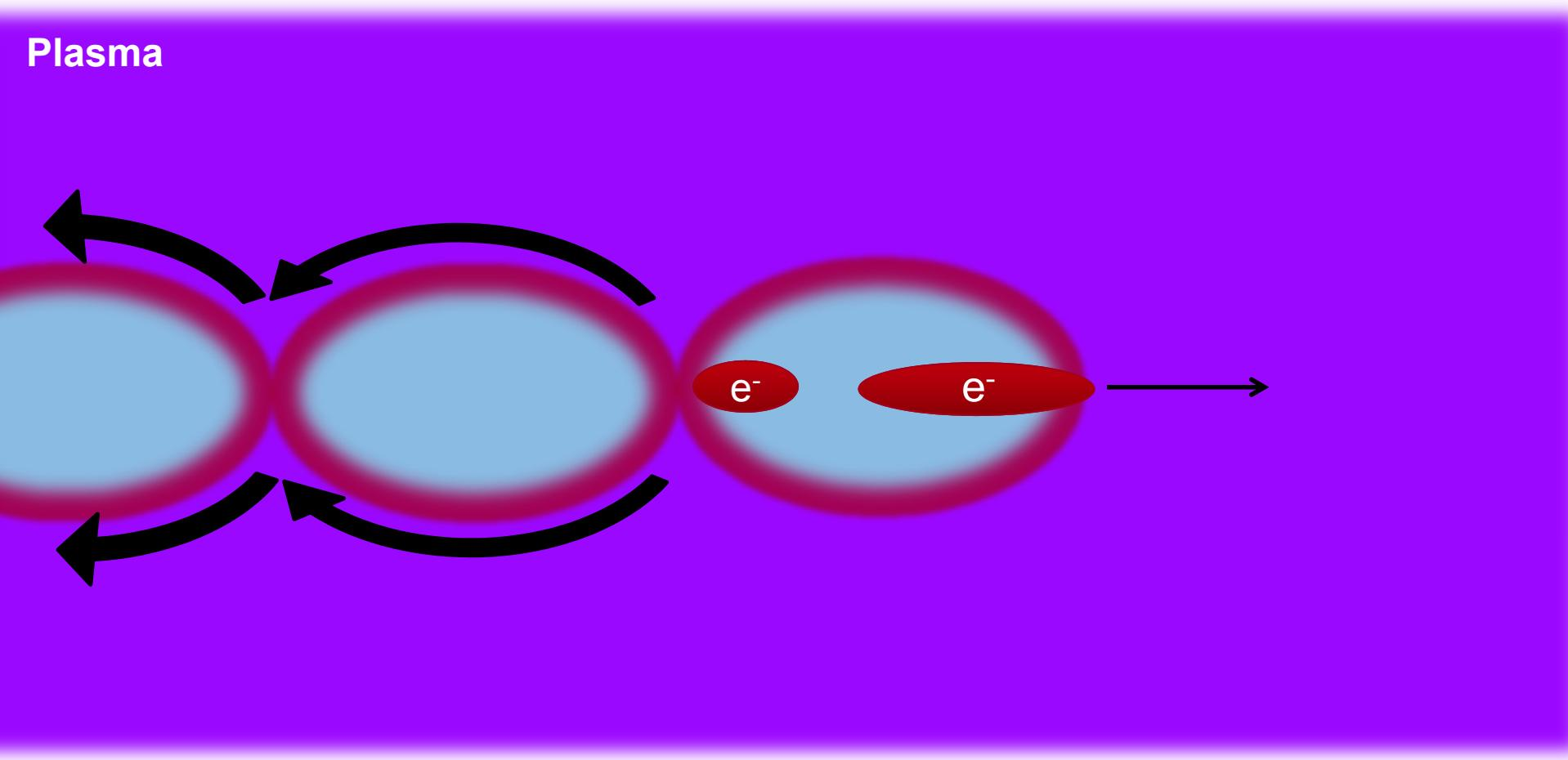
To extract energy from the wakefield, we place a “witness” bunch in the back of the bubble, where it can ride the wake and gain energy.
