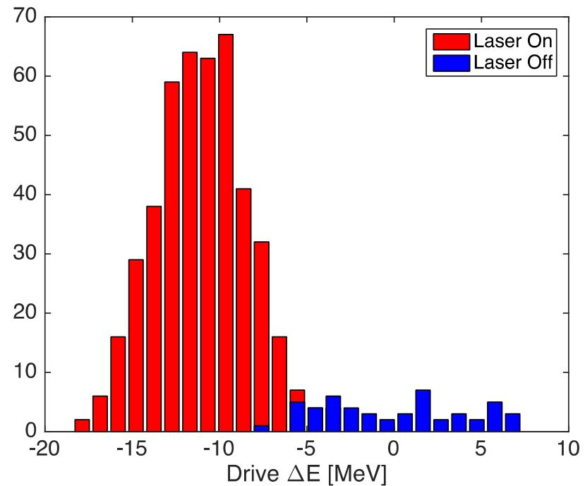
The witness beam gains about 20 MeV on average, while the drive beam loses about 11 MeV, giving a transformer ratio of 1.8.
