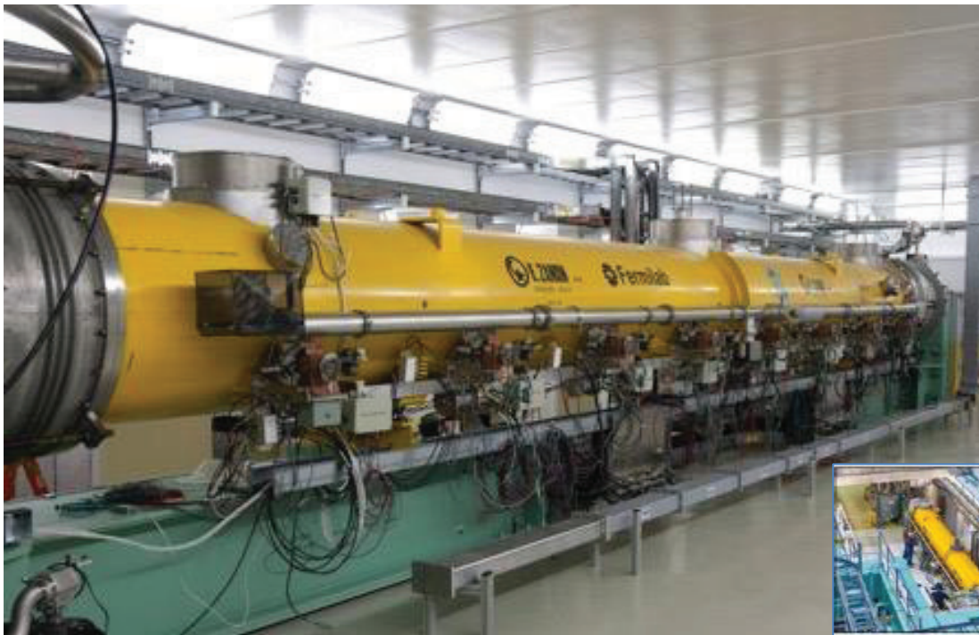
CM2 in its home at Fermilab's SMT building, as part of the future Advanced Superconducting Test Accelerator. (Image credit: Fermilab.)
