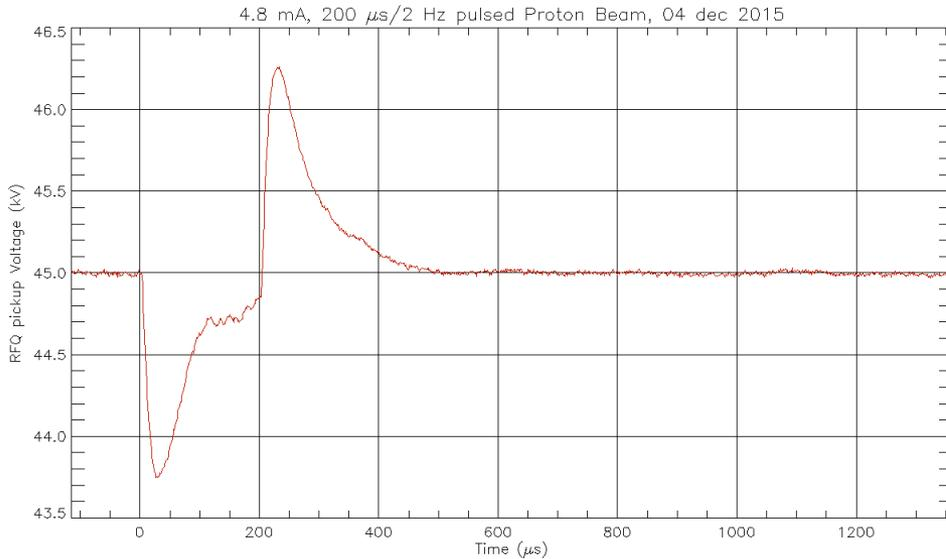
Perturbation of the RF voltage with a 200 $\mu$ s, 5mA pulse of proton
