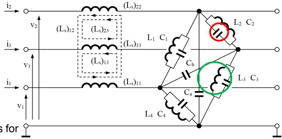
TLM are used to define tolerance requirements for RFQ construction according to the tuner position
