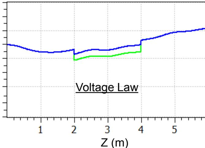
RF voltage law used as input for beam dynamics calculations
