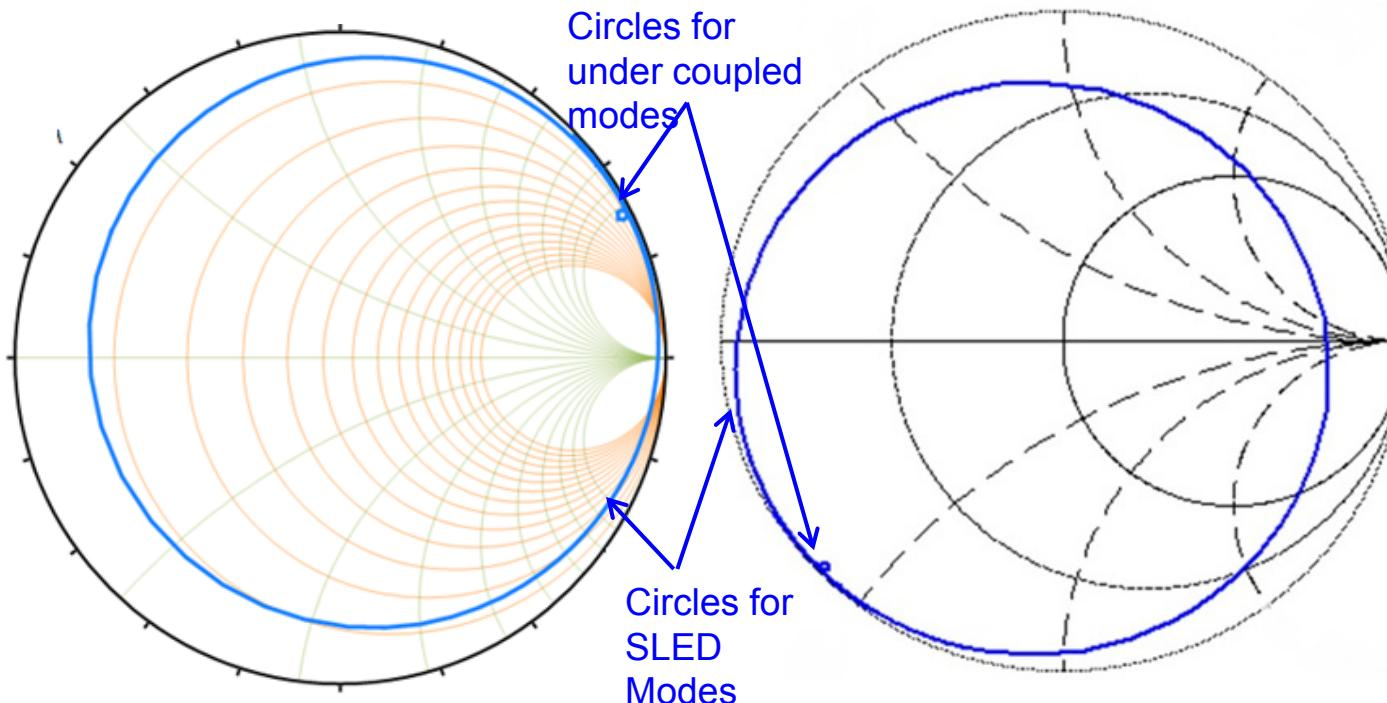
Smith Chart for Theoretical Design Simulation Showing Both SLED Working Modes and Next Mode.
