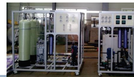
DI water system (completed)
