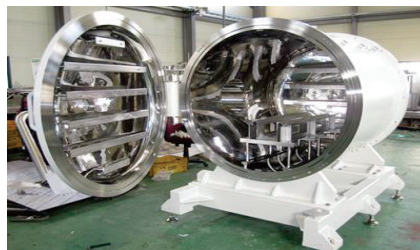
Vacuum Furnace (completed)
