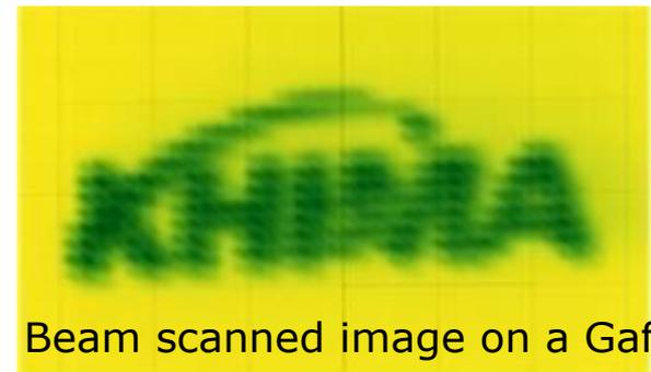
Beam scanned image on a Gaf film
