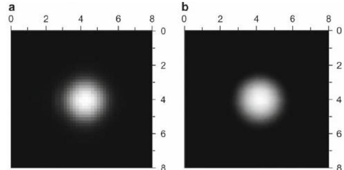
Beam spot image at profile monitor
