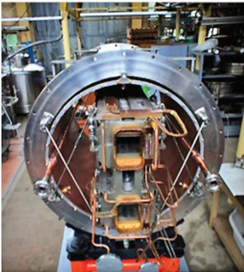
Figure 2: Double-aperture superconducting dipole magnet of the NICA Collider.
