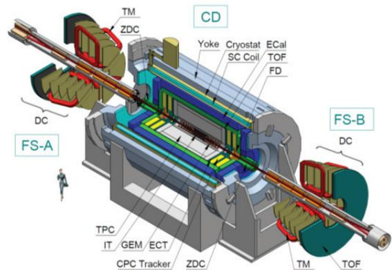
Figure 3: The MPD experimental set-up view.
