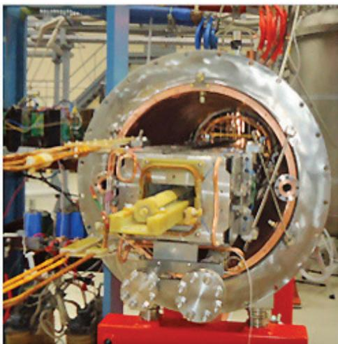
Figure 12: The Booster dipole magnet during the cold tests and magnetic field measurements.
