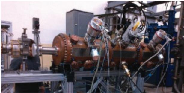
Figure 8: RFQ linac with RF, vacuum components and laser ion source in Nuclotron injector's hall at JINR.
