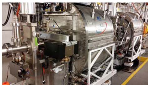
Figure 2: RF cavities C and D in the storage ring tunnel.
