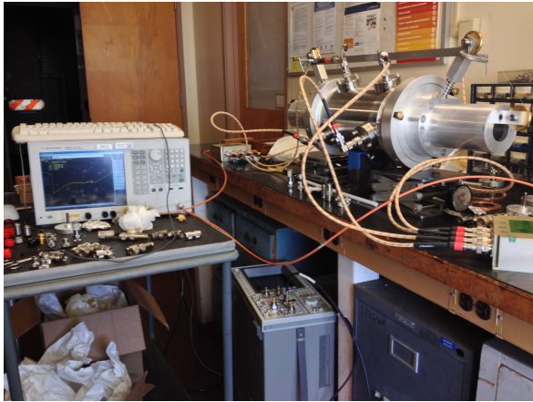
Figure 2: Cavity undergoing RF bench tests.
