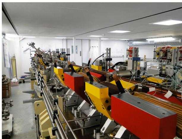
Figure 5: Installation of the vacuum vessel string on the first girder.
