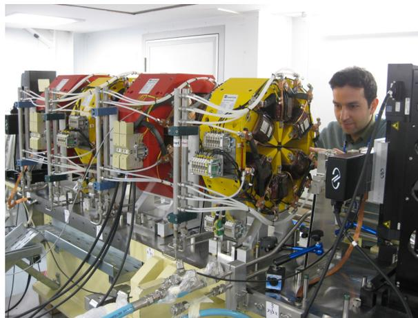
Figure 2: Alignment of a group of multipole magnets using the stretched wire method.
