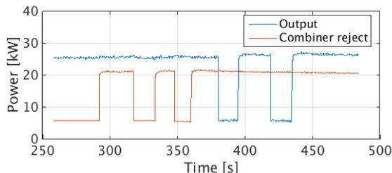
Figure 7: Power steps of output and reject channels.
