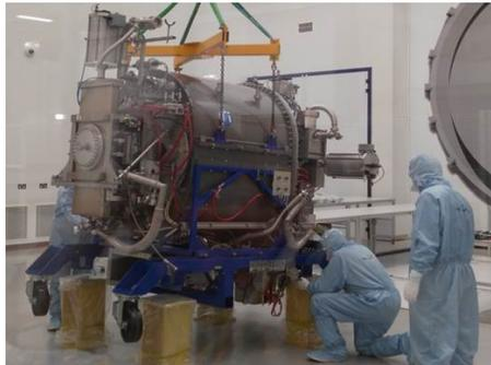
Figure 3: Cavity window change in cleanroom.
