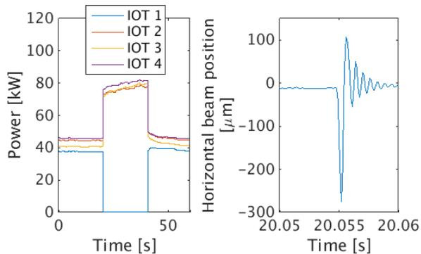
Figure 8: Reaction of remaining IOTs to the loss of power from one IOT (left) and the effect on stored beam (right).
