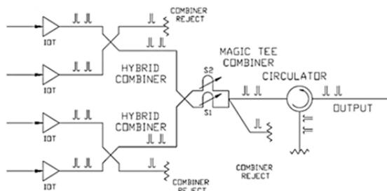
Figure 6: IOT combination scheme.
