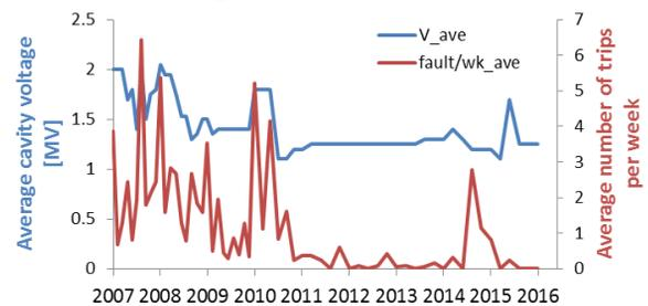
Figure 2: Average cavity operating voltage (blue) and frequency of cavity fast vacuum trips (red).
