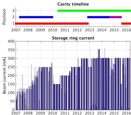
Figure 1: Storage ring current (below) and cavity arrangement in the RF straight (above).
