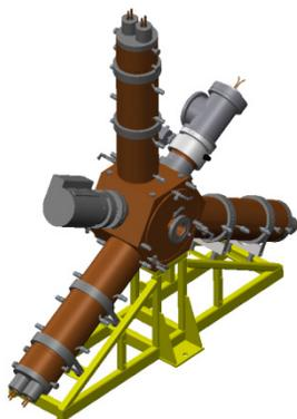
Figure 4: EU HOM-damped cavity.
