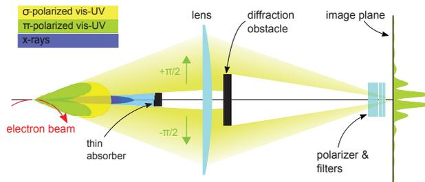
Figure 4: Schematic of the obstacle diffractometer technique.
