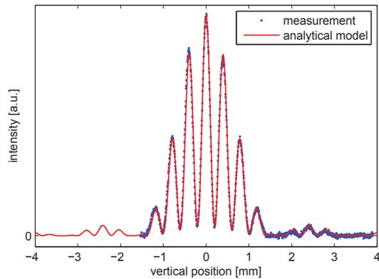
Figure 6: Vertical profile from a double-slit ( $d = 6.2$  mm,  $2a = 1.5$  mm) at 488 nm wavelength. Measurement (blue dots) and analytical calculation (red line). The vertical beam size is  $10.5 \mu\text{m}$ .
