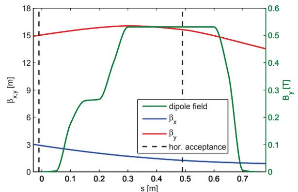
Figure 2: Design beta functions and dipole field strength in the matching dipole. The dashed lines mark the maximum horizontal angular acceptance of the diagnostic beamline.
