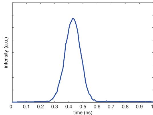
Figure 8: Longitudinal bunch profile measured at  $<1$  mA current. The rms bunch length is 55 ps.
