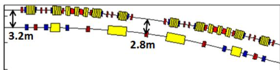
Figure 1: Layout of 1/24 of storage ring (outer) and booster ring (inner).
