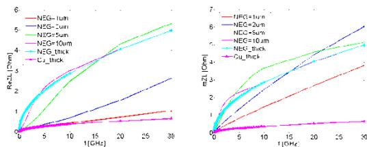
Figure 2: Longitudinal impedance for different thickness of NEG coating (Left: real part, Right: imaginary part).
