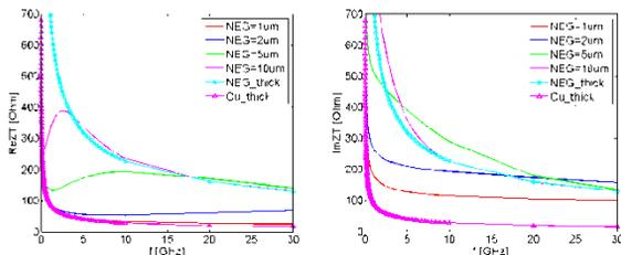
Figure 3: Transverse impedance for different thickness of NEG coating (Left: real part, Right: imaginary part).
