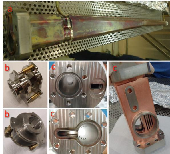
Figure 5: Prototype of Sirius storage ring vacuum system components: (a) dipole chamber, (b) bellows with RF shielding, and (c) pumping station/crotch absorber.
