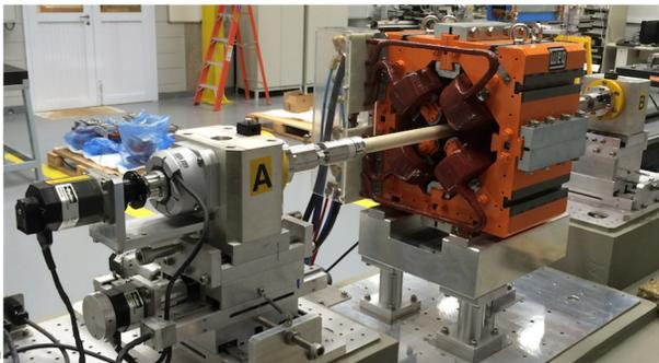
Figure 3: Rotating coil bench.
