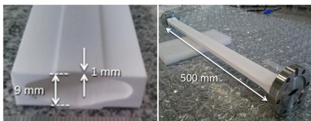
Figure 6: Alumina tube produced in collaboration with ENGECER for the Sirius nonlinear kicker.
