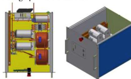
Figure 8: Mechanical design of high power PS modules.
