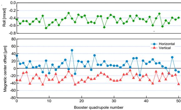
Figure 2: Measured horizontal and vertical magnetic field center and rotation around longitudinal axis for Sirius booster quadrupoles.
