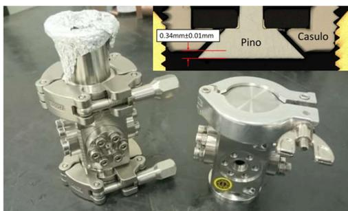
Figure 7: New Sirius storage ring BPM body prototypes. Featured in the corner is a button metallographic section showing good alignment between button and housing.
