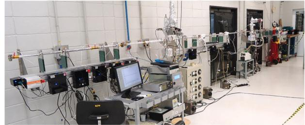
Figure 4: Test assembly of 1/40 of the Sirius storage ring vacuum system.
