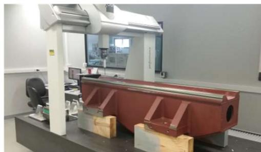
Figure 9: New girder prototype during dimensional measurement.
