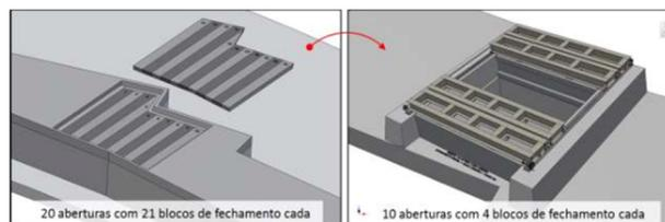
Figure 10: New design for the tunnel roof openings.
