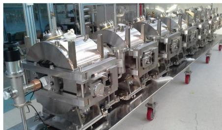
Figure 2: Spoke cavities in one cryomodule.
