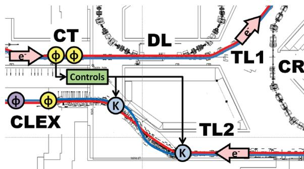
Figure 1: Simplified schematic of the PFF system. Red and blue lines depict orbits for bunches arriving late and early at the first phase monitor,  $\phi$ , respectively. The trajectory through the TL2 chicane is changed using two kickers,  $K$ .
