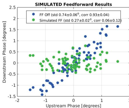
Figure 5: Simulated upstream–downstream mean phase distribution.
