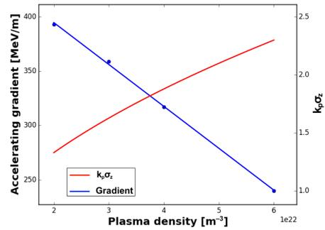
Figure 4: Dependence of average accelerating gradient for particles in the tail of the bunch on plasma density, for a bunch radius of  $50 \mu\text{m}$ . The variation of the product  $k_p \sigma_z$  is also shown, and the gradient plot includes a least-squares fit to a linear function.
