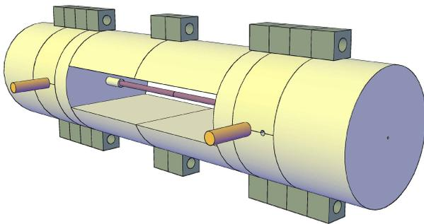
Figure 3: Preliminary design of the housing for the capillary tube.
