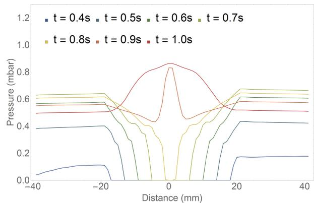
Figure 4: Result of CFD simulation for pressure distribution. Gas inlets are located at edges of the plot, with distance measured from the centre of the capillary.
