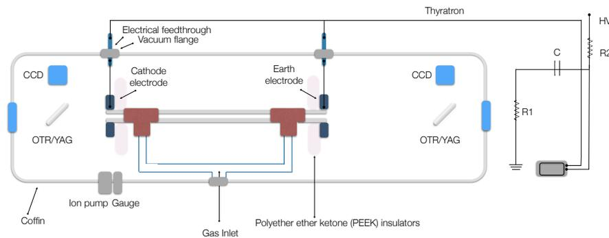
Figure 2: Capillary high voltage plasma discharge source within its vacuum chamber (not to scale).
