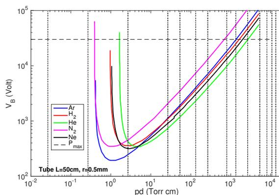
Figure 1: Empirical Paschen's curves for various gases as a function of gas pressure and the distance between the discharge electrodes. Vertical dotted lines denote the conditions given in Table 1 for a 50 cm capillary discharge tube with the radius of 0.5 mm. Horizontal dashed line denotes the limit of the high voltage source. Curves are extrapolated beyond  $pd = 10^3 \text{ Torr cm}$ .
