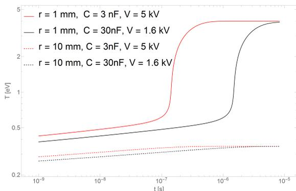
Figure 5: Results of preliminary circuit parameter analysis for electron temperature with time: Low capacitance, high current model (red) and high capacitance/low current model (black).  $r$  is cap radius,  $C$  is capacitance and  $V$  is voltage; scaled so that stored energy is constant.
