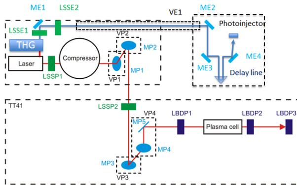
Figure 3: Functional schematic of the laser beam lines to the plasma cell and photoinjector indicating the mirrors (blue) and their surrounding vacuum tanks, the laser safety shutters (green) and laser beam dumps (violet).
