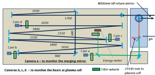
Figure 6: Setup on the optical table downstream the merging chamber with diagnostic equipment allowing monitoring the laser beam profile in the plasma cell. Distances between mirrors are in millimetres.
