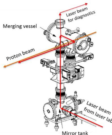
Figure 4: Assembly of mirror tank and merging vessel. The ionizing laser beam arrives in the trench and is directed towards the plasma cell. A small fraction of the beam is coupled out to the diagnostics beam line.
