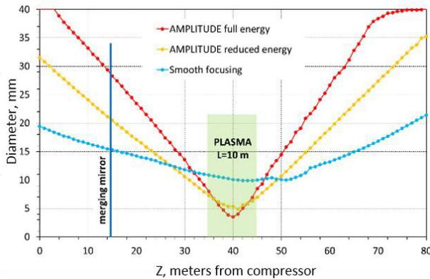
Figure 5: Laser beam diameter at 1% level of maximum.
