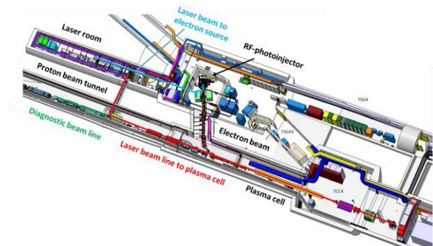
Figure 1: Layout of AWAKE facility with laser beam lines to plasma cell (in red), diagnostics beam line (in green) and to electron source (in blue).
