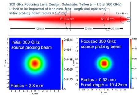
Figure 7: Pre-designed focusing lens for 300 GHz electromagnetic wave.
