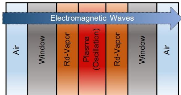
Figure 1: Schematic view of layers for the electromagnetic wave simulation.
