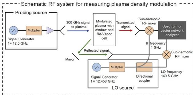
Figure 5: Schematic RF heterodyne system for measuring plasma density modulation.
