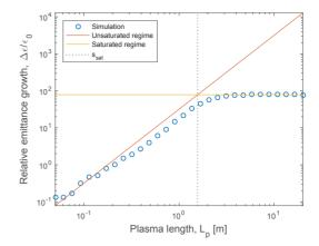
Figure 3: Emittance growth vs. plasma length for a 100 GeV beam with 3 % rms energy spread, normalized emittance 100 nm and an initial offsets of 1  $\mu$ m and 40  $\mu$ rad. Emittance growth is seen to transition from the unsaturated regime (red line) to the saturated regime (yellow line) at the predicted saturation length (dotted line).
