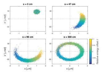
Figure 2: Evolution of the witness bunch in phase space, where colors indicate the relative energy offset. The initial beam, offset by 1  $\mu$ m and 40  $\mu$ rad in x and x' respectively, gets progressively stretched while it traverses the circumference of the offset ellipse (unsaturated regime) until ending up as a steady-state ring (saturated regime).
