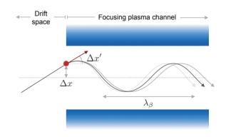
Figure 1: The witness beam enters the plasma channel with a positional offset  $\Delta x$  and angular offset  $\Delta x'$  relative to the drive beam (which defines the channel). Each energy slice then oscillates with wavelength  $\lambda_{\beta}(\gamma) = 2\pi \beta_m(\gamma)$ , resulting in increased projected emittance.
