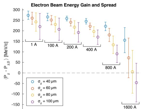
Figure 3: Preliminary beam loading studies [13], showing the energy gain and spread (the error bar) for electron bunches of different lengths and peak currents, accelerated in a pre-modulated proton wake. The results indicate that a peak current of 200–400 A optimally loads the wake for bunch lengths of 40–60  $\mu\text{m}$ .
