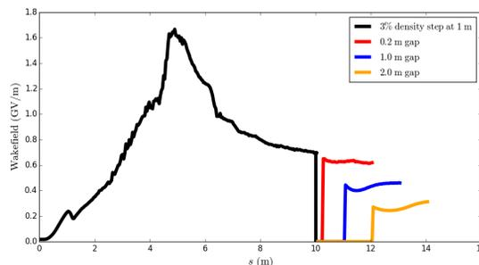
Figure 2: The effect of a plasma interstage on the wakefield amplitude, as function of interstage length, assuming no focusing optics in the interstage. After 1 m of vacuum interstage, the wakefield gradient has decreased by about a factor two.
