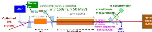
Figure 1: Possible layout for AWAKE Run 2. The proton beam is micro-bunched in the first plasma stage. An electron beam is accelerated in the second plasma stage.
