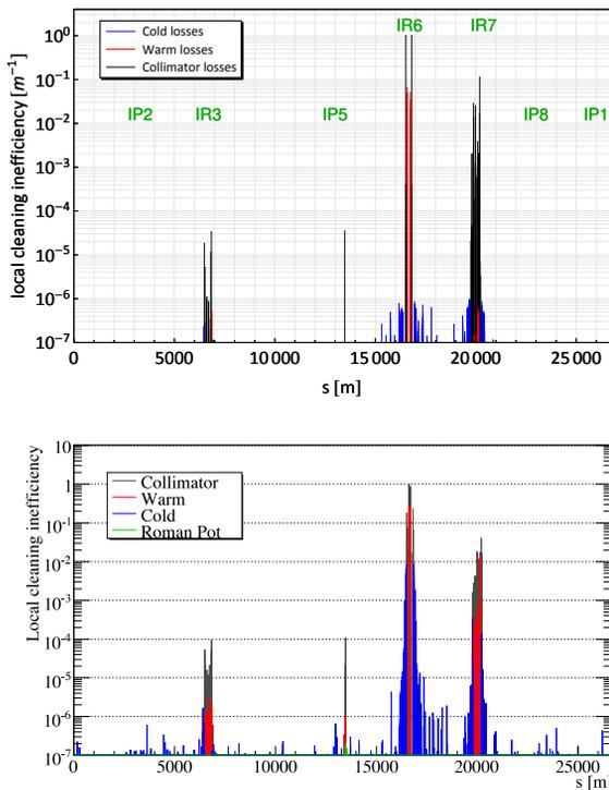
Figure 2: Loss distribution in the ring following asynchronous beam dump at 6.5 TeV with injection optics ( $\beta^* = 11$  m): SixTrack simulation (top) and measurement performed on 6.9.2015 at 10:59:13 (bottom).
