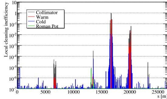
Figure 3: Loss distribution in the ring following asynchronous beam dump at 6.5 TeV with squeezed optics ( $\beta^* = 80$  cm): SixTrack simulation (top) and measurement performed on 4.7.2015 at 15:42:24 (bottom).
