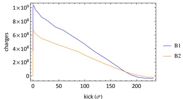
Figure 1: Abort gap population, measured by the abort gap monitors during the asynchronous dump test with tight collimator settings and  $\beta^* = 80$  cm for both beams, giving as a function of total kick in  $\sigma$  summed over all MKDs.
