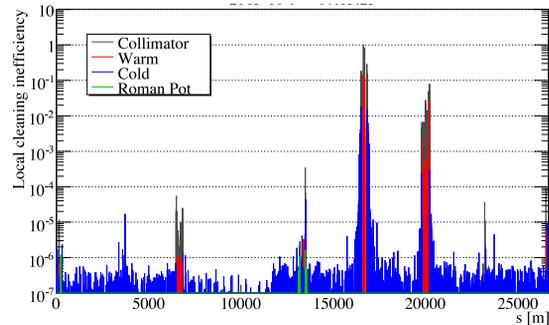
Figure 4: Loss distribution in the ring following asynchronous beam dump at 6.5 TeV with squeezed optics ( $\beta^* = 80$  cm) and tighter TCT settings in IP1/5: SixTrack simulation (top) and measurement performed on 9.10.2015 at 07:13:25 (bottom).
