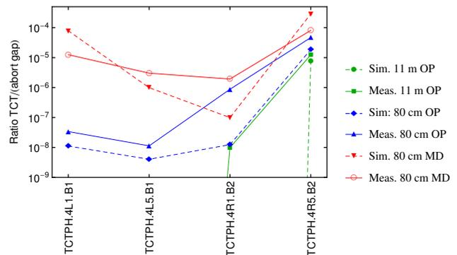
Figure 5: Fraction of the total abort gap population impacting on the TCTs in IR1/5 during the asynchronous dump in simulation and measurement for the cases discussed.
