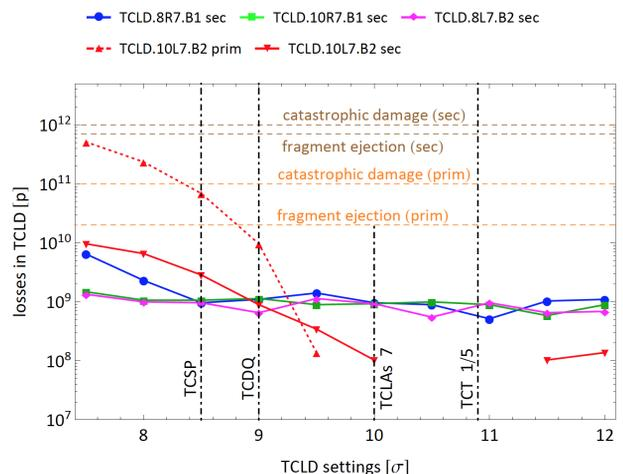
Figure 3: Simulated losses at TCLDs, following beam dump failure, as function of collimator settings. Nominal TCLD settings are set to the level of the absorbers (TCLA) in IR7. Damage thresholds for tungsten [20] added for comparison.
