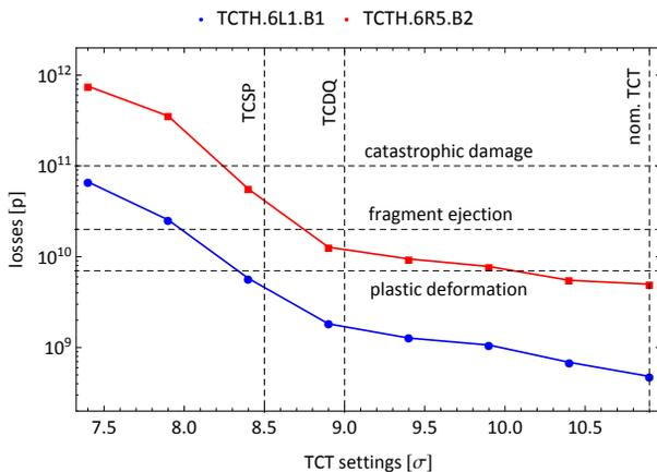
Figure 2: Losses at the most loaded TCT in IP1 and IP5 as function of collimator settings. Damage thresholds [20] are added for comparison.
