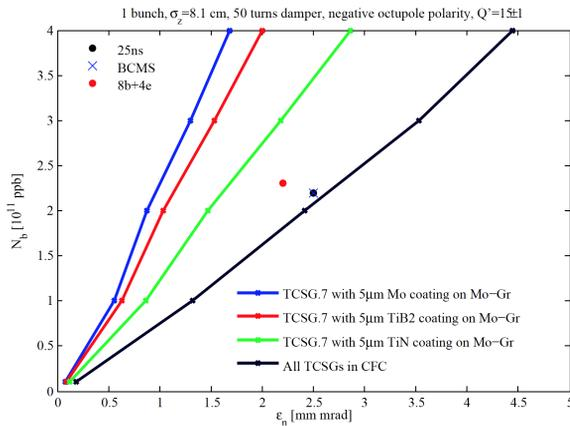
Figure 1: HL-LHC beam stability for different secondary collimator configurations in IR7. Note that the stability area is on the right of each curve.
