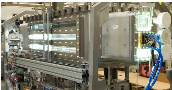
Figure 4: Assembly of HRMT-23 experiment allocating the three full collimator jaws.
