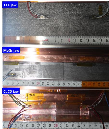
Figure 5: Collimator jaws after being tested in HRMT-23.
