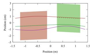
Figure 1: Trajectories in the LER cell for the design energies. Magnet locations (red for F, green for D) are also shown.
