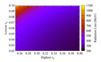
Figure 7: Synchrotron radiation loss per particle as a function of maximum horizontal and minimum vertical tune.
