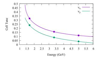
Figure 3: Tune as a function of energy in the LER arc cell. Points are the values for the design energies.
