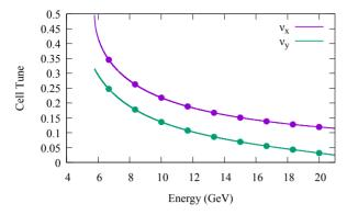
Figure 4: Tune as a function of energy in the HER arc cell. Points are the values for the design energies.
