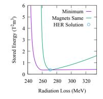
Figure 6: Boundary for minimum stored energy and radiation loss solutions. The violet line is the minimum for fixed maximum horizontal and vertical tunes. The green line is the boundary when the transverse magnet structure is constrained to be the same. The circle is our chosen solution for the HER.
