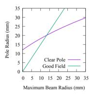
Figure 9: Magnet pole radius as a function of maximum beam radius in the midplane. The violet line is what is required to keep the beam 12 mm from the pole, and the green line is to keep the beam at 2/3 the pole radius.
