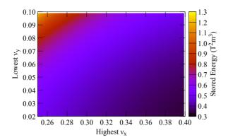
Figure 8: Magnetic stored energy as a function of maximum horizontal and minimum vertical tune.
