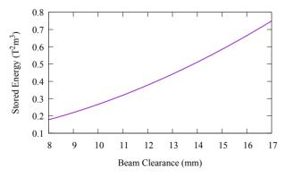
Figure 10: Magnetic stored energy as a function of the required distance to the pole.
