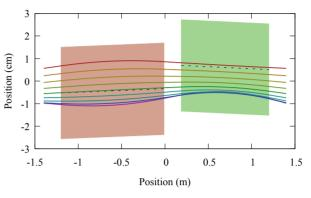
Figure 2: Trajectories in the HER cell for the design energies. Magnet locations (red for F, green for D) are also shown.
