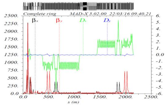
Figure 5: Beta and dispersion functions around the JLEIC ion collider ring after correction.
