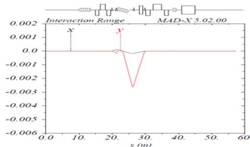
Figure 3: Closed orbit in the IR of the JLEIC ion ring.
