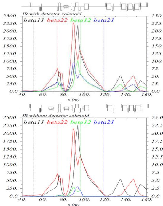
Figure 4: Local compensation of the coupling effect caused by the detector solenoid in the JLEIC ion collider ring (top: without compensation, bottom: with compensation).
