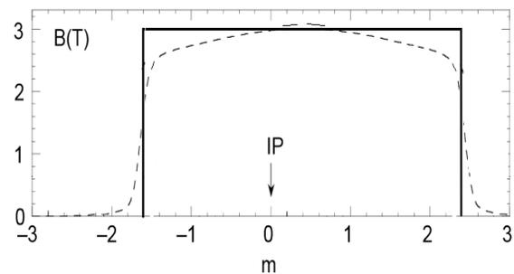
Figure 2: Hard edge model of the detector solenoid.
