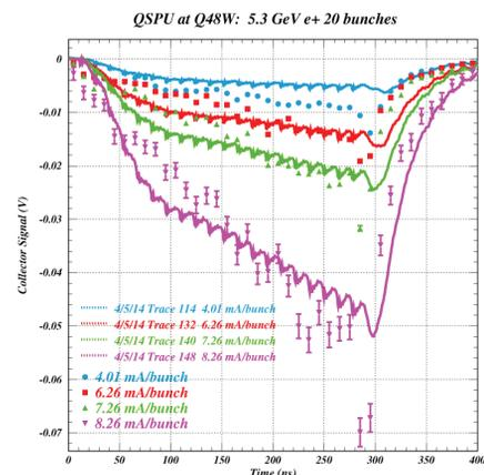
Figure 1: Comparison of modeled to measured electron detector signals for a train of 20 bunches of 5.3-GeV positrons with populations varying from  $6.4 \times 10^{11}$  to  $13.2 \times 10^{11}$  (4.01 to 8.26 mA/bunch).
