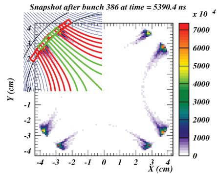
Figure 4: Effect on the cloud profile shown in Fig. 3 given by raising the bunch population from  $11.6 \times 10^{11}$  to  $13.2 \times 10^{11}$ . The red lines show the increased acceptance given by augmenting the present electron detector with two adjacent detectors.
