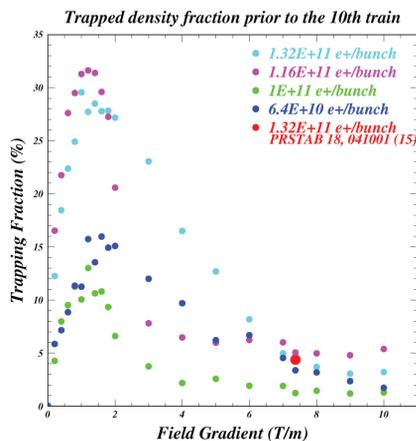
Figure 7: Dependence of the modeled cloud trapping fraction on the quadrupole magnetic field strength for bunch populations ranging from  $6.4 \times 10^{11}$  to  $13.2 \times 10^{11}$ .
