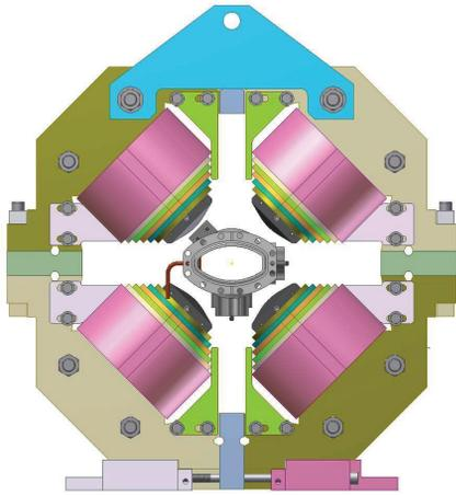
Figure 6: Schematic drawing of the vacuum chamber installed in the quadrupole magnet.
