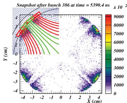
Figure 3: Modeled cloud profile at the end of the second beam revolution, i.e. following  $2 \times 183$  bunch spacings for the case of  $11.6 \times 10^{11}$  bunch population. The insert shows the position of the vacuum chamber wall and the field lines of the quadrupole magnetic field. The green lines show the hole diameter and the positions of the rows of holes which allow cloud electrons to reach the stripline detector.
