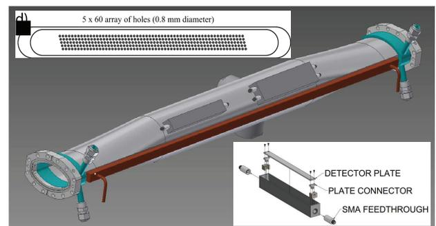
Figure 5: Schematic drawing of the new instrumented vacuum chamber design. The insets show the layout of the hole array for one of the three detectors, the enclosure for which is shown on the lower right.
