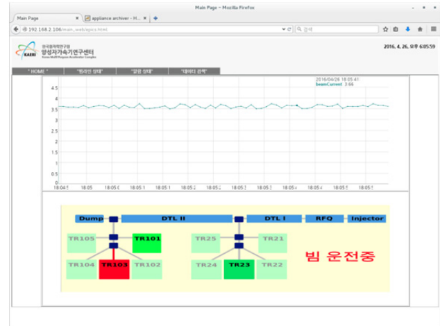
Figure 4: Beam current and status monitoring system using WebSocket based Process Data Access (WebPda) with Glassfish WebSocket server
