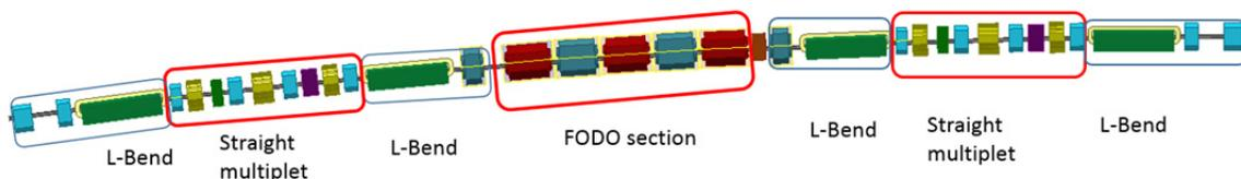
Figure 1: Magnet distribution in one cell.
