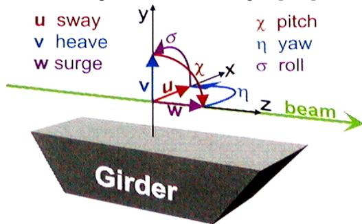
Figure 7: The definition of coordinates of the girder (This figure is borrowed from [3, 5]).
