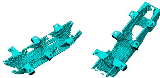
Figure 4: Topological optimization of 6-axes girder body. Left: structural, Right: modal.
