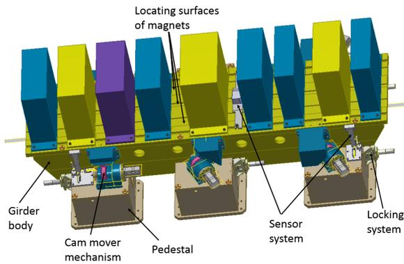
Figure 2: 6-axes girder system.
