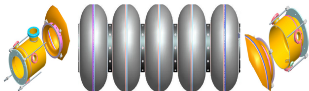
Figure 5: Ridge waveguide prototype measurement setup (top) and detachable copper BNL4 cavity.
